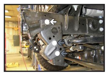
6a. **All Models:** Using a 16MM socket, remove the bolt holding the frame bracket (white).
