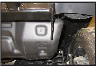
12. Trim belly pan for baseplate clearance in one of two ways listed below then reinstall belly pan. **Note:** For Sport, Sport S, and Overland models the skid plate will need to be reinstalled before thebelly pan.
