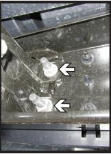
Using an 18MM socket, remove the four (4) nuts holding the bumper to the frame. Do this on both sides of the vehicle. Remove the bumper and set aside to be reinstalled later.
