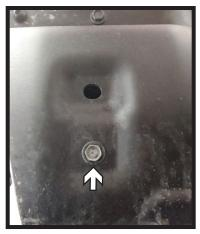
2b. **Rubicon w/Steel Bumper Models:** Using an 13MM socket, remove the seven (7) bolts from the belly pan. There are five (5) bolts along the front edge (left and center) and two (2) in the back (right). Remove belly pan and set aside to be reinstalled later.
