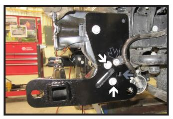
9a. Rubicon w/Steel Belly Pan Models: Place the belly pan bracket between the frame and the baseplate. Install the two (2) existing 10MM bolts (white). Then install the one (1) 1/2" bolt with hardware into the bottom back hole (gray). May need to ream out the bottom back hole. Mojave Models Only: Install the one (1) existing 6MM bolt (black). Do this on both sides of the vehicle.
