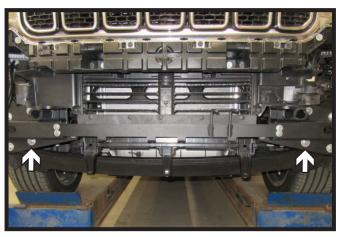
14. Install two (2) 1/2" x 1-1/2" bolts with flat washers and nylon lock nuts into the bottom inside holes on the front of the vehicle.
