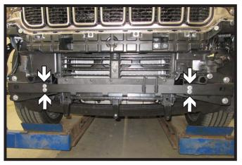
10. Attach cross member to baseplates, start four (4) 3/8" x 1" bolts with flat washers and nylon lock washers. Ensure baseplate is level and tighten baseplate on each side then cross member.
