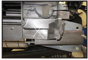
Using a utility knife, trim plastic shroud as shown on both sides of the vehicle and remove piece.
