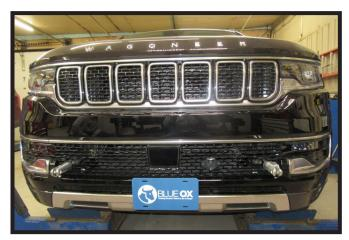
17. Hold the fascia as close to its original position, mark and trim the fascia around the convenience links and attachment tabs. Reinstall the fascia.
