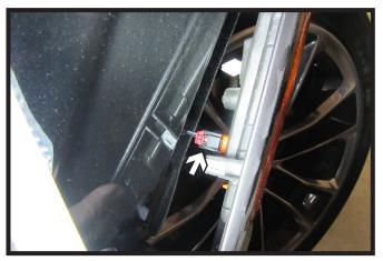
Unsnap the wheel well trim past the fascia joint. Unplug light as trim is pulled back. Place soft cloth between trim and vehicle to hold trim out of the way. Do this on both sides of the vehicle.
