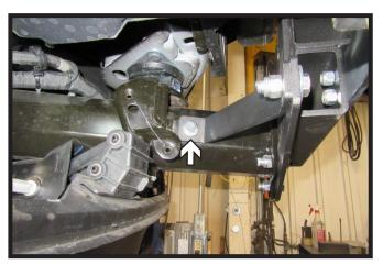
13. Install one (1) 1/2" bolt with lock washer and whiz nut. Do this on both sides of the vehicle.
