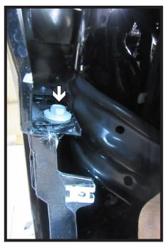
3. Pull back the wheel well liner. Using a 10MM socket, remove the one (1) bolt from the fascia joint. Do this on both sides of the vehicle.
