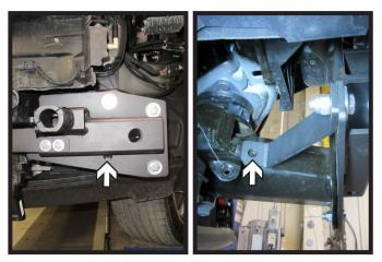
13. Using a 1/2" drill bit, drill the bottom inside hole on the front of the baseplate (left). Then using the support bracket as a template, drill 1/2" hole in frame (right). Do this on both sides of the vehicle.
