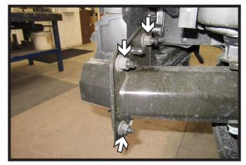
7. Using a 18MM socket or wrench, remove the three (3) nuts from the bumper. Do this on both sides of the vehicle. Remove bumper, it will not be reinstalled.
