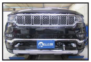
Hold the fascia as close to its original position, mark and trim the fascia around the convenience links and attachment tabs. Reinstall the fascia and reconnect all electrical and hose.
