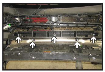
Using a 13MM socket, remove the five (5) nuts on the backside of the fascia. Remove foam piece and set aside. It will not be reinstalled.
