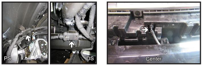
5. Remove fascia and set aside to be reinstalled later. Unplug the electrical on both sides of the vehicle and hose in the center as the fascia is removed.
