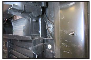
17. Using a utility knife, trim the upper shroud as indicated. Do this on both sides of the vehicle.
