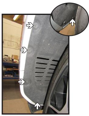
4. Using an 8MM socket, remove the five (5) bolts from along the edge of wheel well. Do this on both sides of the vehicle.
