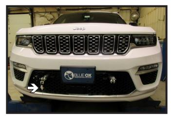
26. Hold the fascia as close to it's original position, mark and trim the fascia around the convenience links and attachment tabs. Reinstall the fascia, fascia cover, and belly pan. Reconnect all electrical connections and windshield washer fluid line.
