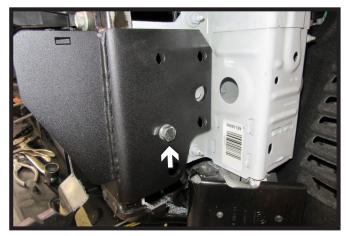
21. Start a 1/2" x 1-1/2" bolt with lock washer and whiz nut in the bottom front hole. Leave loose at this time. Do this on both sides of the vehicle.
