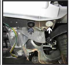
9. Using a 10MM socket, remove the four (4) bolts (white) from the underside of the fascia. Then remove the two (2) push pins (gray).
