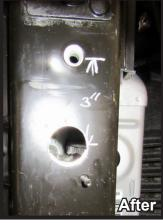
18. Measure 3" from the center of the top hole down. Using a 1-1/4" hole saw, drill hole centering hole with existing holes on the frame and the bottom of the 3" measurement. Do this on both sides of the vehicle.
