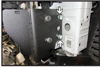
23. Install two (2) 1/2" x 1-1/2" bolts with lock washers and whiz nuts into back holes. Do this on both sides of the vehicle. Tighten all bolts at this time.
