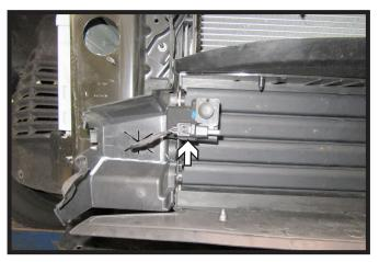
15. Remove the temperature sensor and feed through the plastic on the passenger side of the vehicle. Place out of the way during baseplate installation, it will be reinstalled later.
