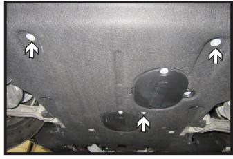
8. Using a 10MM socket, remove the three (3) bolts from the belly pan. Let belly ban hang.
