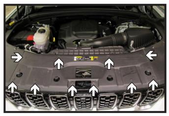
Remove the ten (10) push pins from the top of the fascia cover. Remove fascia cover and set aside to be reinstalled later.
