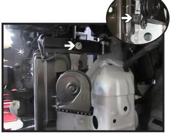
13. Unclip horn from the bracket (inset). Then using a 10MM socket, remove the one (1) bolt. Place the horn out of the way during baseplate installation, it will be reinstalled later. Do this on both sides of the vehicle.
