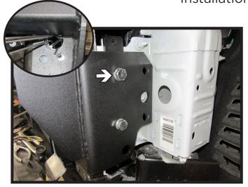
22. Insert spacer plate at top of baseplate between the frame and baseplate with the slotted end facing downward. Once spacer plate is in position insert 1/2" x 1-1/2" bolt with lock washer and whiz nut into top front hole (inset). Do this on both sides of the vehicle.
