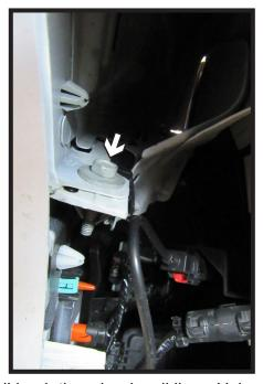
5. Pull back the wheel well liner. Using a 10MM socket, remove the one (1) bolt from the fascia joint. Do this on both sides of the vehicle.
