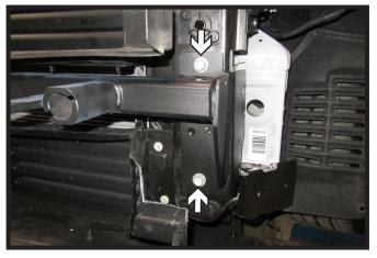
19. Hold baseplate into place on the vehicle frame and start the existing bolts in both front holes. Do this on both sides of the vehicle.
