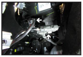
11. Unplug two (2) electrical connections on the driver side of the vehicle. Remove fascia and set aside to be reinstalled later.
