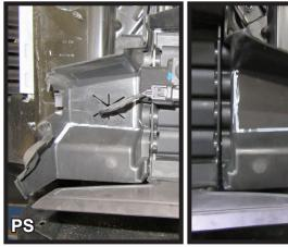
16. Using a utility knife, trim the shroud on each side of the bottom shutters as indicated.
