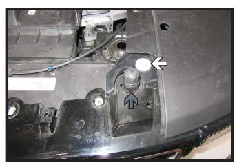
Using a 10MM socket, remove the one (1) bolt from the top of the fascia. Do this on both sides of the vehicle. Then turn hood bumper (gray) a quarter of a turn and remove.
