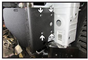
20. Using 1/2" drill bit, drill the four (4) holes on the side of the frame using the baseplate as a template. Do this on both sides of the vehicle.
