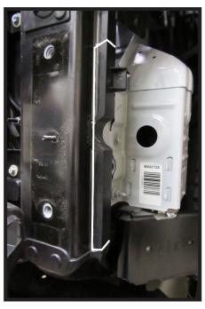
14. Using a reciprocating saw, trim the frame as shown. Do this on both sides of the vehicle.
