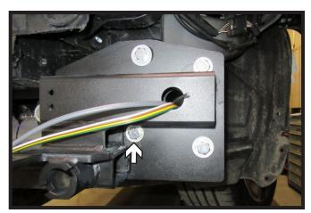
17. Install one (1) 1/2" x 1-1/2" bolt with flat washer and nylon lock nuts into the bottom inside hole on the front of the baseplate. Leave loose at this time. Do this on both sides of the vehicle.
