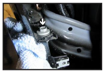
3. Pull back the wheel well liner. Using a 10MM socket, remove the one (1) bolt from the fascia joint. Do this on both sides of the vehicle.
