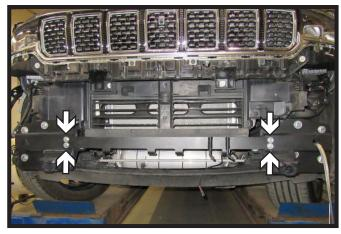
18. Attach cross member to baseplates, start the four (4) 3/8" x 1-1/4" bolts with flat washers and nylon lock washers. Ensure baseplate is level and tighten baseplate on each side then cross member.
