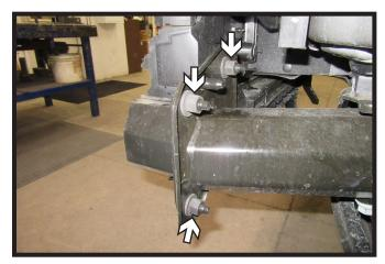
7. Using an 18MM socket or wrench, remove the three (3) nuts from the bumper. Do this on both sides of the vehicle. Remove bumper, it will not be reinstalled.
