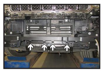
19. Attach plastic piece from bumper to cross member using four (4) 1/4" x 1" bolts with flat washers and lock washers.
