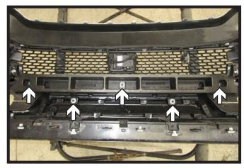
Remove the five (5) clips from the foam piece on the back of the fascia. Remove foam piece and set aside, it will not be reinstalled.
