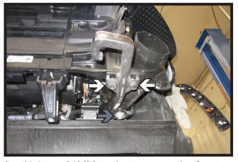
6. Using a 21MM socket, remove the front two (2) bolts (white) on the tow hooks. Then using an 18MM socket, remove the back one (1) bolt (gray). Remove tow hook, it will not be reinstalled. Reinstall back bolt from tow hook (gray). Do this on both sides of the vehicle.
