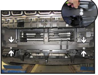
16. Pull back plastic shroud (inset) and attach cross member to baseplates, start the four (4) 3/8" x 1-1/4" bolts with flat washers and nylon lock nuts. Ensure baseplate is level and tighten baseplate on each side then cross member.
