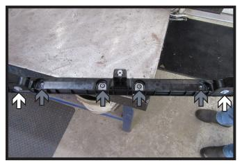
10. Using a 10MM socket, remove the two (2) bolts (white) from the plastic piece on the bottom of the bumper. Then using a 1/4" drill bit, drill out the four (4) plastic rivets (gray). Remove plastic piece and set aside to be reinstalled with the baseplate.
