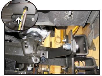
13. Using a 1/2" drill bit, drill the bottom inside hole on the front of the baseplate (inset). Then using the support bracket as a template, drill 1/2" hole in frame (white). Do this on both sides of the vehicle.
