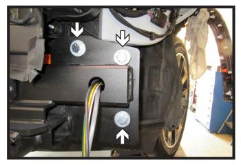
11. Hold baseplate in place and start the three (3) 1/2" x 1-1/2" bolts with flat washers and nylon lock nuts. Snug up the baseplate into place but leave loose. Do this on both sides of the vehicle.
