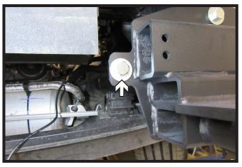
12. Attach support bracket to baseplate using one (1) 1/2" x 1-1/2" bolt with flat washer and nylon lock nut. Do this on both sides of the vehicle.
