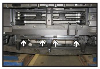
17. Attach plastic piece from bumper to cross member using four (4) 1/4" x 1" bolts with flat washers and nylon lock nuts.
