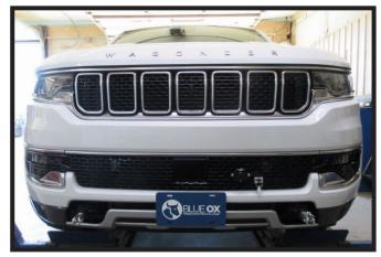
Hold the fascia as close to its original position, mark and trim the fascia around electrical rods. Reinstall the fascia and reconnect all electrical connections.
