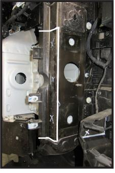
15. Using a reciprocating saw, trim the frame as shown. Do this on both sides of the vehicle.
