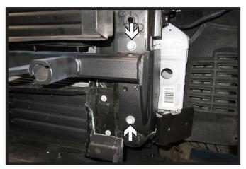
22. Hold baseplate into place on the vehicle frame and start the existing bolts in both front holes. Do this on both sides of the vehicle.
