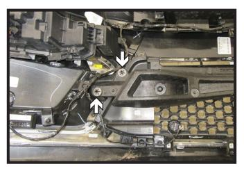
20. On the back side of the fascia, remove the four (4) clips, two (2) on each side, from the foam piece. Remove foam piece, it will not be reinstalled.
