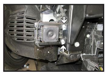
30. Reinstall the pedestrian alert system onto the bracket on the passenger side of the vehicle using the existing bolts and hardware.
