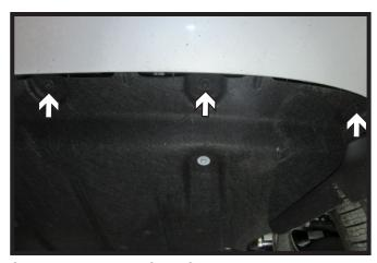
6. Using an 8MM socket, remove the five (5) bolts from the bottom of the fascia.
