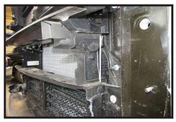
18. Using a utility knife, trim the upper shroud as indicated. Do this on both sides of the vehicle.
