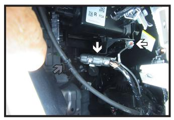
Unplug two (2) electrical connections (white) on the passenger side of the vehicle. Then disconnect windshield washer fluid line (gray).
