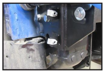
29. Install clips from pedestrian alert bracket onto the tabs on the passenger side of the baseplate.
