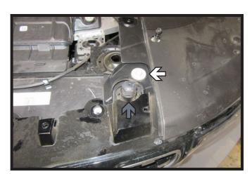
3. Using a 10MM socket, remove the one (1) bolt from the top of the fascia. Do this on both sides of the vehicle. Then turn hood bumper (gray) a quarter of a turn and remove.
