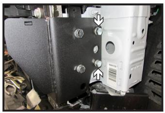
26. Install two (2) 1/2" x 1-1/2" bolts with lock washers and whiz nuts into back holes. Do this on both sides of the vehicle. Tighten all bolts at this time.
