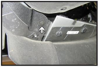
7. Using an 8MM socket, remove the one (1) bolt on the underside of the fascia in front of the tire. Do this on both sides of the vehicle.
