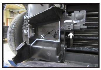
16. Remove the temperature sensor and feed through the plastic on the passenger side of the vehicle. Place out of the way during baseplate installation, it will be reinstalled later.
