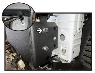
25. Insert spacer plate at top of baseplate between the frame and baseplate with the slotted end facing downward. Once spacer plate is in position insert 1/2" x 1-1/2" bolt with lock washer and whiz nut into top front hole (inset). Do this on both sides of the vehicle.
