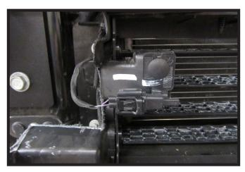
28. Reinstall the temperature sensor on the passenger side of the vehicle. Then reinstall the horns on both sides of the vehicle.
