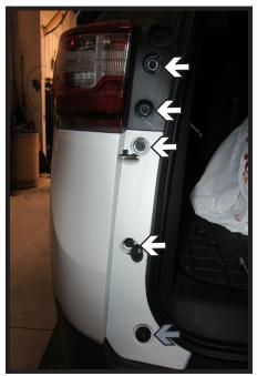
Unpop the covers for the five (5) bolts on the back panel of the vehicle. Then using a 7MM socket, remove the four (4) top bolts (white) and use a T20 Torx to remove the one (1) bottom bolt (gray). Do this on both sides of the vehicle.
