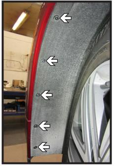
3. Using a T15 Torx, remove the five (5) bolts along the edge of the wheel well. Do this on both sides of the vehicle.
