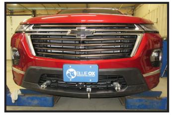
23. Hold the fascia as close to its original position, mark and trim the fascia around the convenience links and attachment tabs. Reinstall the fascia, fascia cover and reconnect all electrical.
