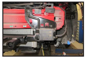
20. Reinstall the ACC bracket on the driver side of the vehicle.
