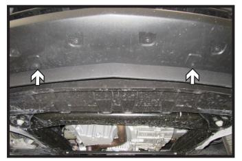
7. Using a T15 Torx, remove the two (2) bolts from the underside of the fascia.
