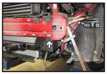
14. Slide baseplate into place. Use large vise grips to hold baseplate in place. Then using a 3/8" drill bit, drill hole in frame using baseplate as a template. Do this on both sides of the vehicle.
