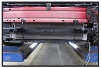
22. Reinstall metal rods to the front of the vehicle.
