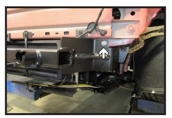
14. Install one (1) 3/8" x 1-1/4" bolt with lock washer and lock nut. Do this on both sides of the vehicle. Remove vise grips.
