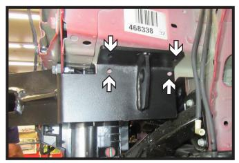
15. Using a 3/8" drill bit, drill the remaining four (4) holes on the side of the vehicle using the baseplate as a template. Do this on both sides of the vehicle.
