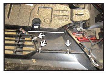
12. Remove the three (3) push pins from the back side of the fascia. Zip tie wire loom straight across below the foam piece.
