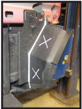
10. Using a utility knife, trim the shutter housing as shown on each side of the vehicle.
