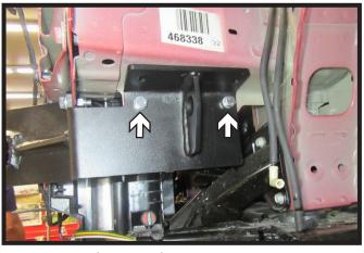
Install 3/8" x 1-1/4" bolts with lock washers and lock nuts into bottom two (2) holes.
