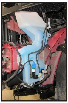
Reinstall the windshield washer fluid reservoir on the driver side of the vehicle and reconnect all lines.
