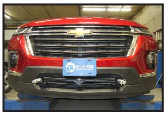
20. Hold the fascia as close to its original position, mark and trim the fascia around the convenience links, attachment tabs and electrical rods. Reinstall the fascia, fascia cover and reconnect all electrical.
