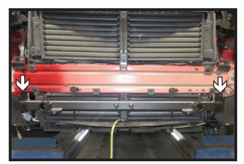
13. Slide baseplate into place. Use large vise grips to hold baseplate in place. Then using a 3/8" drill bit, drill hole in frame using baseplate as a template on each side of the vehicle.
