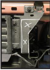
11. Using a utility knife, trim the shutter housing as shown on each side of the vehicle.
