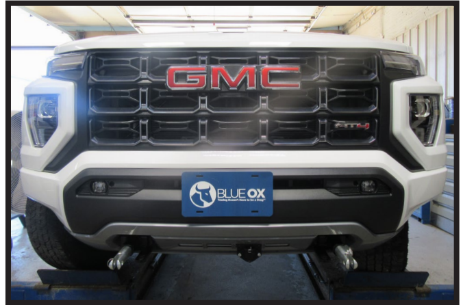
10b. GMC Canyon Models: Reinstall the belly pan, skid plate, fascia, and reconnect all electrical connections.
