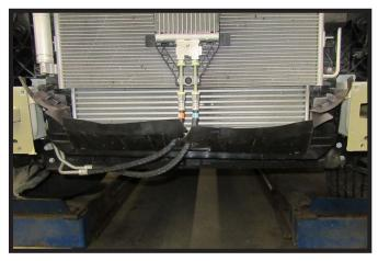
9. Unsnap and remove the plastic shroud from the bottom of the radiator.
