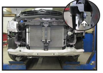
18. Reinstall the ACC Bracket by snapping bottom to the bumper and reinstalling existing bolts into the top two (2) holes with three (3) 1/4" washers on each bolt (inset). Reconnect electrical to ACC sensor.
