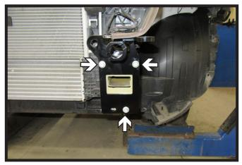
12. Line the inner edge of the baseplate with the inner frame edge. Start the front three (3) 8MM bolts. Tighten but do not apply Loctite Red at this time.
