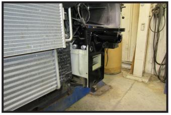
16. Remove the three (3) bolts from the front of the baseplate. Do this on both sides of the vehicle.
