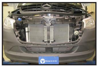
5. Unsnap and remove grille from fascia. Set grille aside to be reinstalled later.
