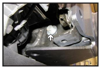
3a. **Baseplates Made Prior to (4/14/23)**: Install the two (2) 1/2" bolts with flat washer and lock washer, one (1) on each side of the frame. Do this on both sides of the vehicle.
