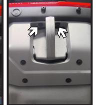
1b. Raptor Models: Remove the seventeen (17) push pins from plastic bumper cover. Pull on area around tow hooks to unsnap cover and remove. Set cover aside to be reinstalled later.
