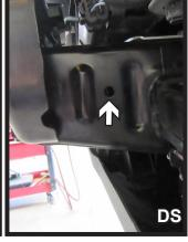
4. Using a 1/2" drill bit, drill out hole on the out side of the frame. Do this on both sides of the vehicle.
