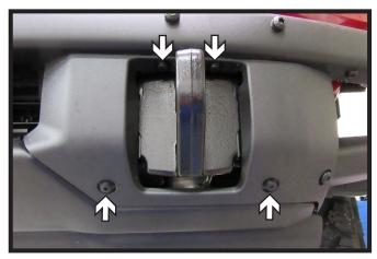
1a. Most Models: Remove the four (4) push pins from plastic tow hook cover. Unsnap cover and remove. Set cover aside to be reinstalled later. Do this on both sides of the vehicle.
