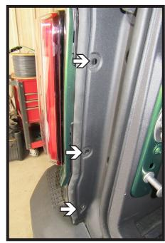
1. Using a Phillip's screw driver, remove the three (3) push pins. Unsnap black plastic piece. Do this on both sides of the vehicle.
