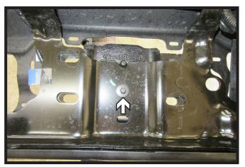
Using an 8MM socket, remove the one
