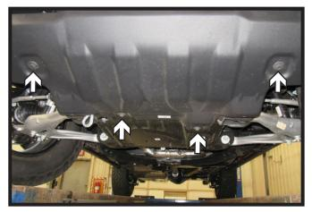
Using a 15MM socket, remove the four
