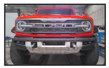
9c. Reinstall belly pan. Hold tow hook cover as close to its original position, mark and trim the covers as needed. Reinstall bumper cover.
