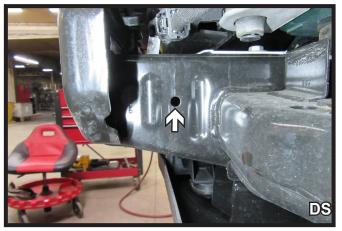
5. Using a 1/2" drill bit, drill out hole on the out side of the frame. Do this on both sides of the vehicle.
