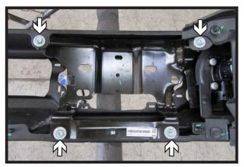
Using a 13MM socket, remove the four
