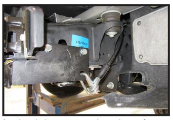
cables to the provided convenience link on the baseplate. The photo above shows the recommended installation of the cables to frame of vehicle. Additional options may interfere with suggested mounting; in this case, secure the cables to a solid piece of the frame as described in the General Information sheet. Be sure the safety cables do not rub against any hoses or moving parts. Do this on **BOTH** sides of the vehicle.
