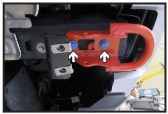
Using a 15MM socket, remove the two
