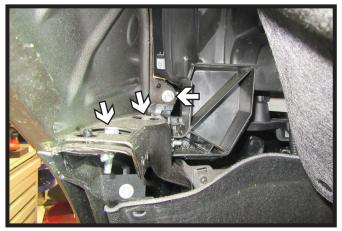
Pull the liner back, then using a 10MM socket remove the three (3) bolts. Do this on both sides of the vehicle.
