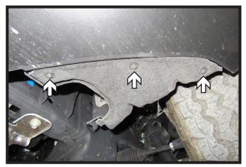
Using a 5.5MM socket, remove the three
