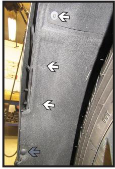
Using a 5.5MM socket remove the three
