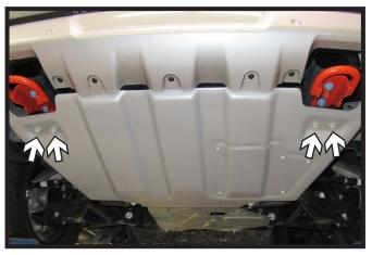
Using a 13MM socket, remove the four (4) bolts from the belly pan, two (2) on each side.
